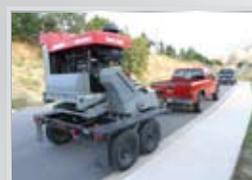
**Transports On Its Own Tandem Axle Trailer** behind a one ton pickup truck.
