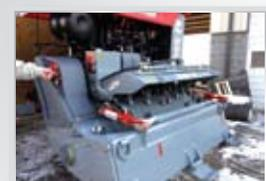
**Top Opening Bit Hatch** opens hydraulically for easy and safe bit inspection and replacement.
