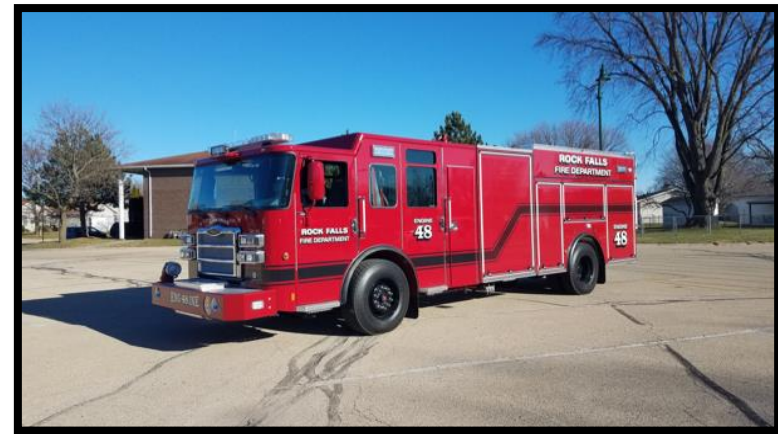
Rock Falls FD Engine 48 - 2020 Pierce Enforcer pumper; 1,500GPM Waterous pump; 750 gallons of water and 30 gallons of foam w/ CAFS system, clean cab concept and pump enclosed panel
