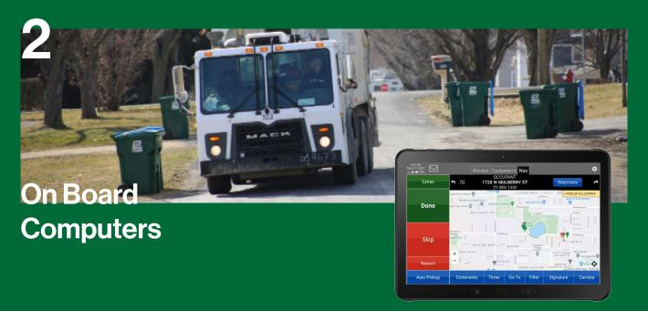
All of our trucks come equipped with these tablets mounted in them for the drivers use. Primarily they are used as a form of communication from the driver back to dispatch communicating what has been done and what has yet to be done. The driver is able to mark extra trash and many other events that may come up. These tablets also provide turn-by-turn navigation for drivers unfamiliar with a route, in the case of a substitute driver.
